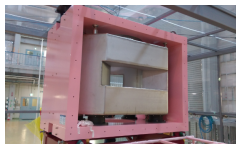
Photo of the Helmholtz magnet for field measurement
