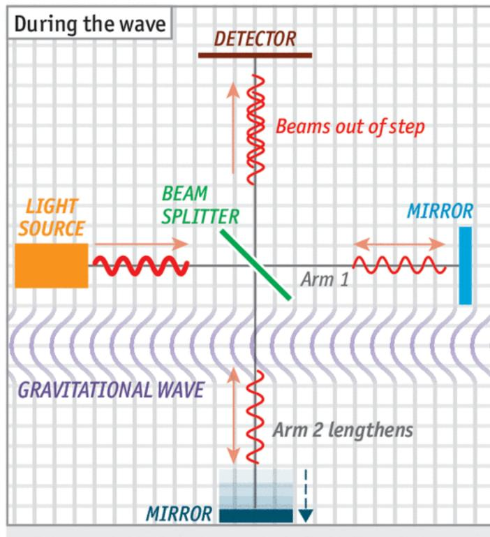
When a gravitational wave arrives, it disturbs spacetime, lengthening (in this example) the light's path along **arm 2**; when the **beams** recombine and arrive at the **detector**, they are no longer in step.
