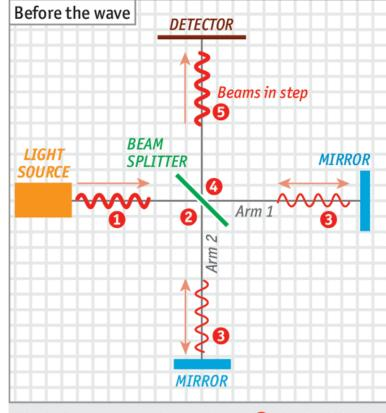
The light source sends out a beam 1 that is divided by a beam splitter 2. The half-beams produced follow paths of identical length (3), reflecting off mirrors to recombine 4, then travel in step to the detector 5.
